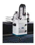
**TCS – Taper Control System –** allows the user to achieve the highest accuracy parts by angling and rotating the inherent waterjet taper "away" from the part straight edge. The TCS uses two additional axes of motion—angular and rotational—to maximize part edge quality and wall straightness. The result is a final part that is produced faster and with straighter walls, regardless of the thickness or composition of the material being cut.
