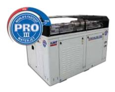
**Upgrade to 90,000 psi** – waterjet cutting with ultra-high pressures of 90,000 psi offers users the latest technology to maximize cutting speeds. For example, 90,000 psi cutting of 1" aluminum is 15-2 ipm while 60,000 psi cutting of 1" aluminum is 5 -10 ipm. With the latest technology from KMT in high pressure seals, cylinders and check valves, operating costs of the 90,000 psi operation have never been lower, and usually cost only a few dollars more per hour than a 60,000 psi operation.
