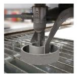
**Automatic Touch Probe and Collision Sensor Bracket** – automatic step touch probe can be programmed at certain distance intervals to engage and insure proper nozzle tip stand-off height control and then adjusted while cutting to compensate if the work piece material is warped or not flat. The collision sensor ring can detect most crashes of the nozzle into tipped-up parts, or other items, via a circular metal ring around the nozzle tip which is pneumatically engaged and easily reset.
